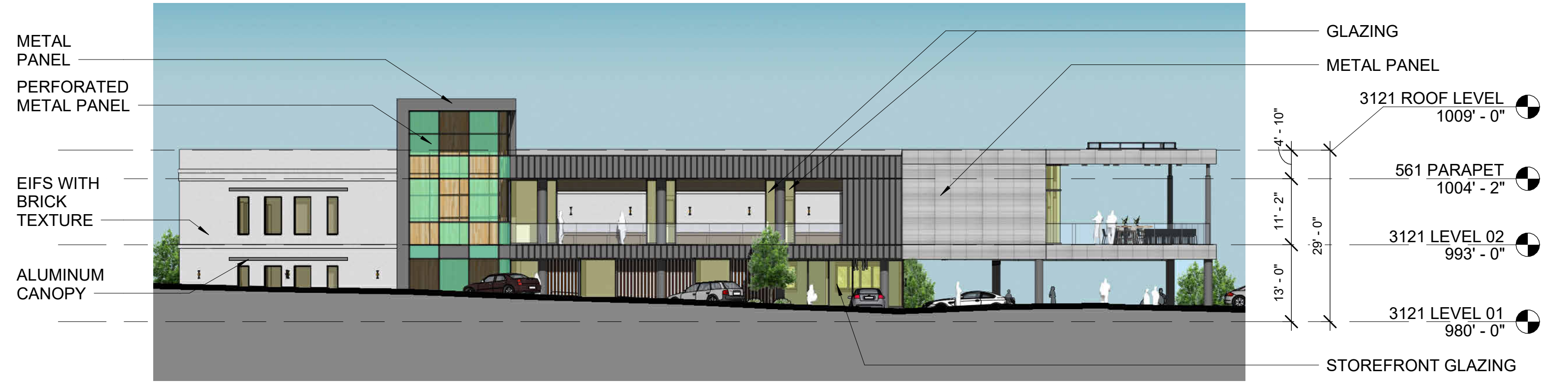
3 NORTH ELEVATION - INTERNAL 1/16" = 1'-0"
