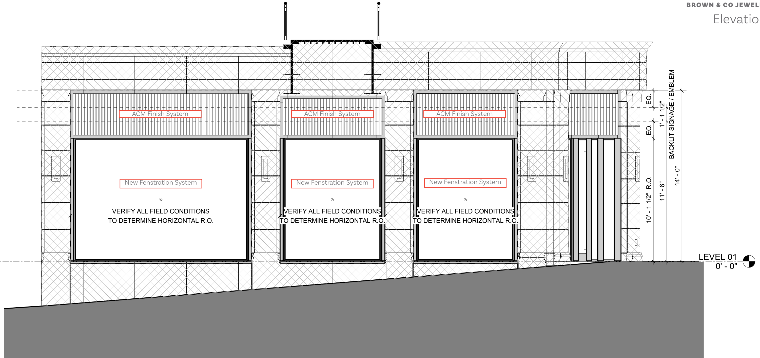
1 Proposed South Elevation (Fenstration Replacement)
