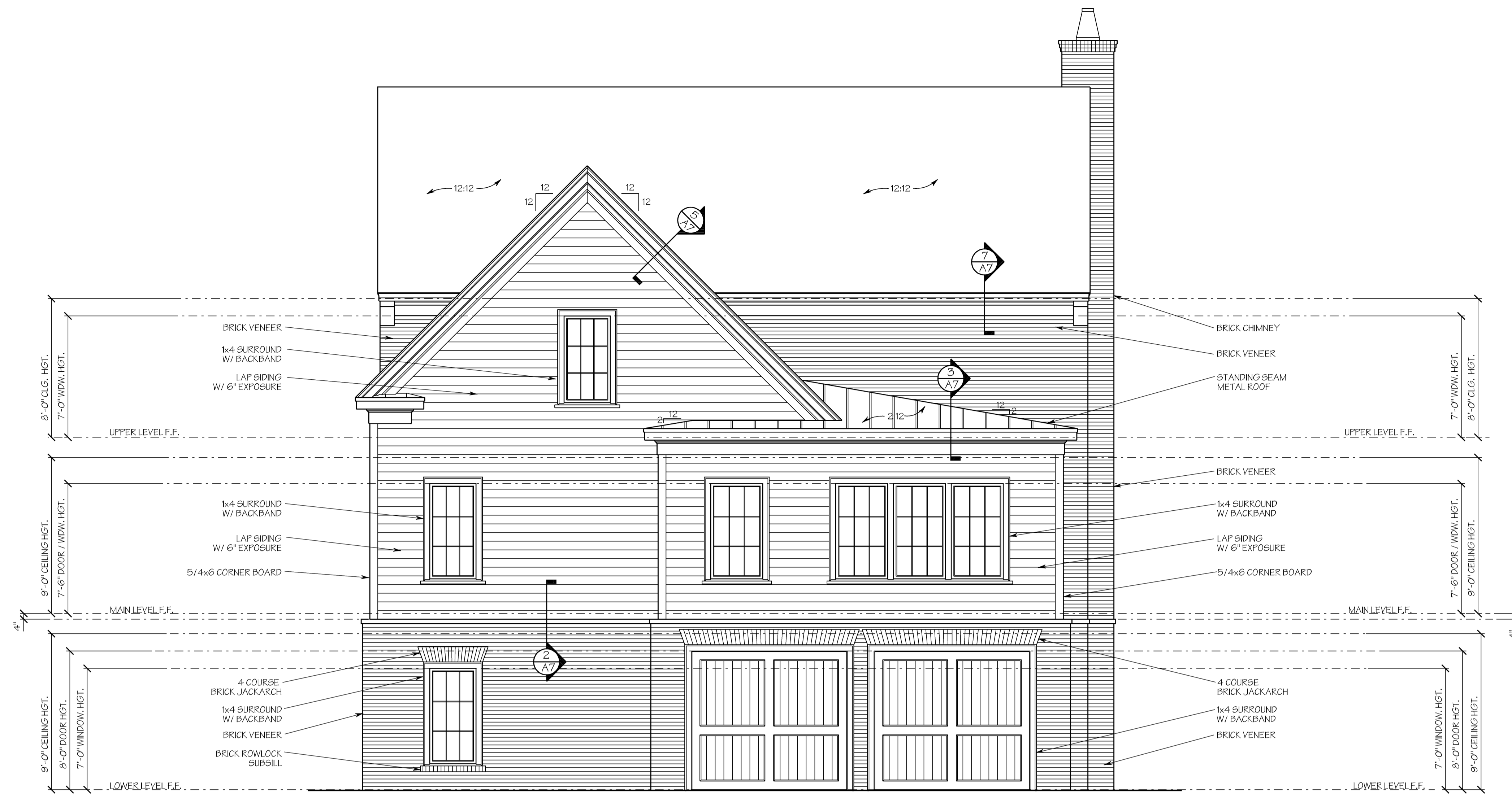
2 REAR ELEVATION SCALE: 1/4" = 1'-0"
