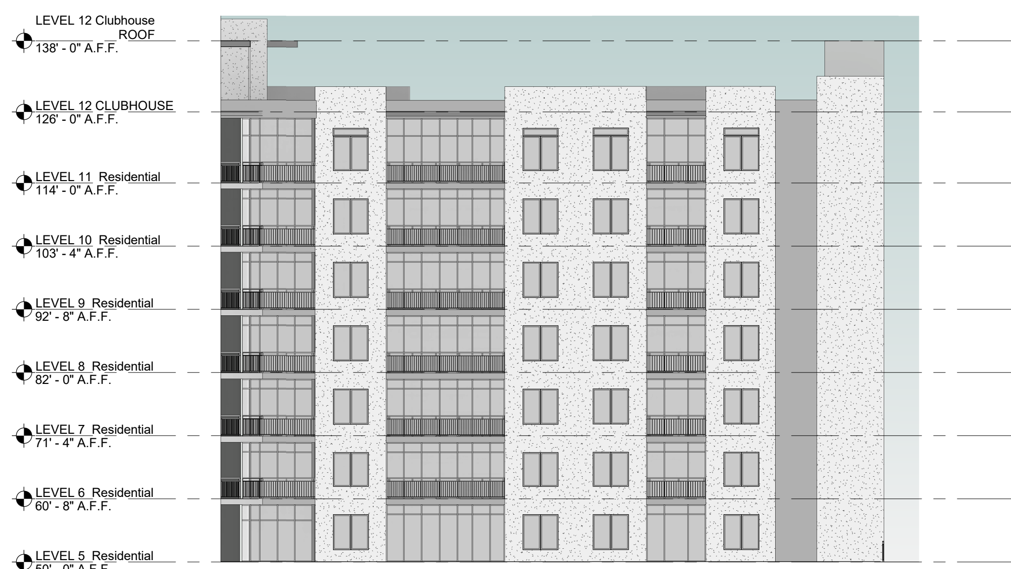
6 PARTIAL EAST ELEVATION (AMENITY DECK) SCALE: 1/16" = 1'-0"
