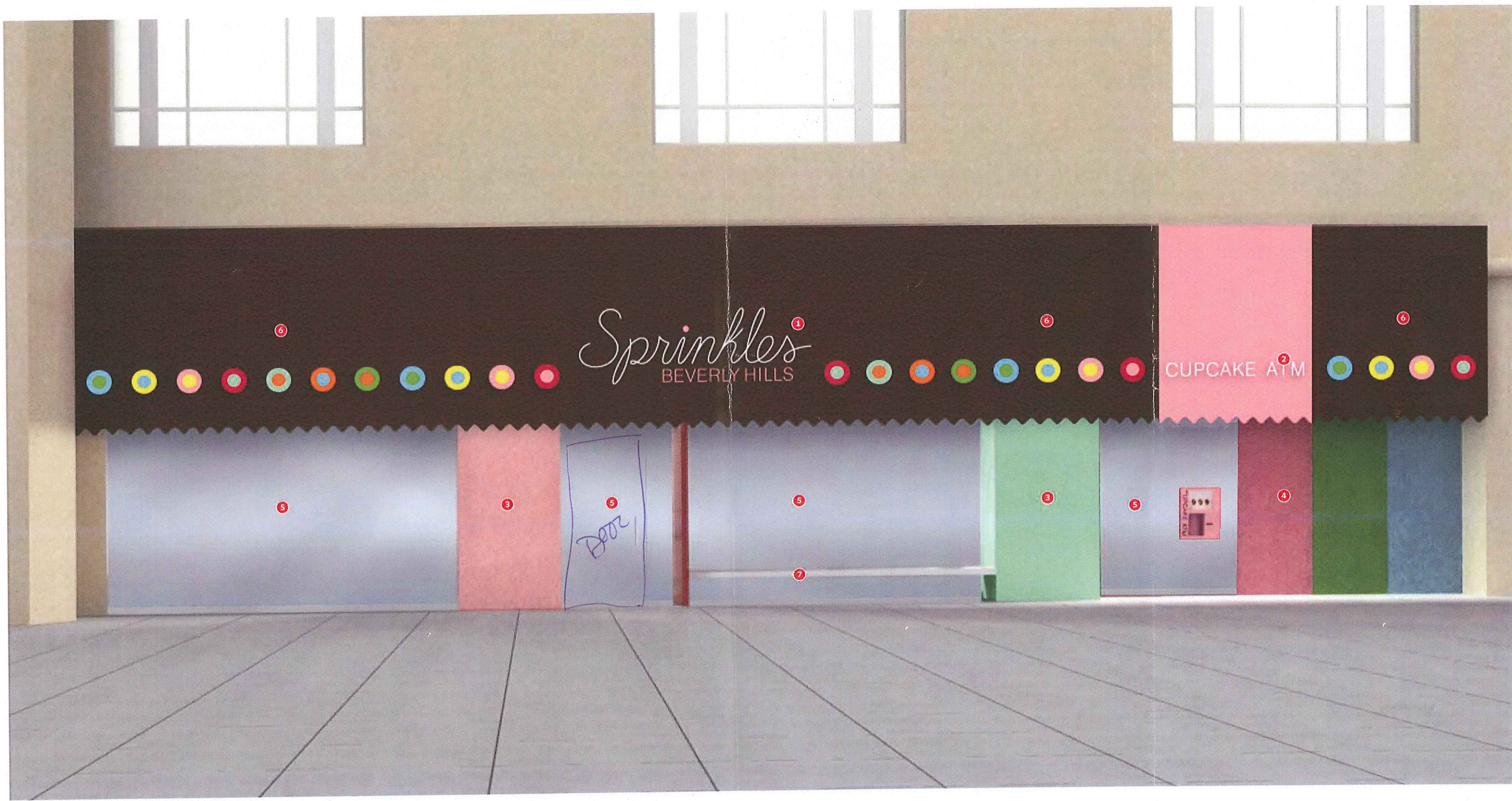
1 primary exterior business identification sign (see page 5) 2 cupcake atm business identification sign (see page 6) 3 perforated metal cladding over EIFS pier wall 4 perforated metal, powdercoated, over EIFS wall 5 tempered glass storefront 6 metal awning with scalloped edge, powdercoated 7 cantilevered bench
